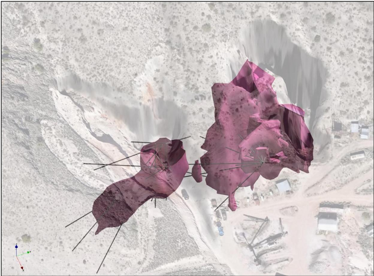
Figure 10.11 shows the preliminary 3-D rendering of the breccia body, which hosts fluor spar mineralization distribution after completion of 2020 delineation drilling at the Lost Sheep Mine, see buildings for scale.
